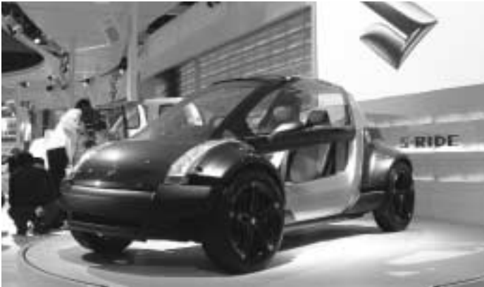
Suzuki S-Ride - an active commuter concept vehicle with motorcycle-like driving (2 seats in tandem)
